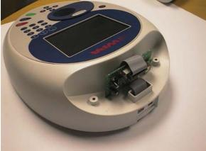
5. Note the slots in the base of the case. The two lugs on the Bluetooth module plug into these
