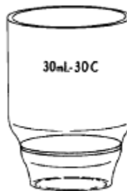
Figure 1. Crucible (C represents the pore size of the crucible). During method development, the analyst will often need to choose an appropriate size for the filtrate and precipitation/digestion used.
