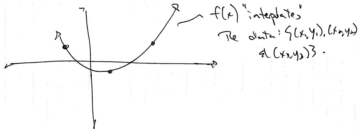
**Definition** The function  $y = P(x)$  (interpolates) the data:  $(x_1, y_1), \dots, (x_n, y_n)$  if  $P(x_i) = y_i \quad \forall 1 \leq i \leq n$ .
