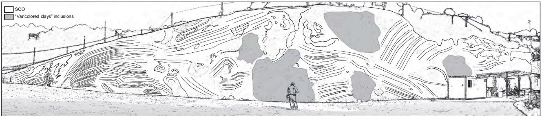
Figure 5. Stratigraphic contact between Stilo-Capo d'Orlando (SCO) Formation and overlying varicolored clays ( 38^{\circ}24'32.64''\text{N} , 16^{\circ}25'38.33''\text{E} ). For location, see Figure 2. The outcrop shows the lowermost section of the varicolored clays with coherent blocks of varicolored clays enclosed within reworked mélange with a clastic fabric and intraclasts from the underlying Stilo-Capo d'Orlando turbidites.
