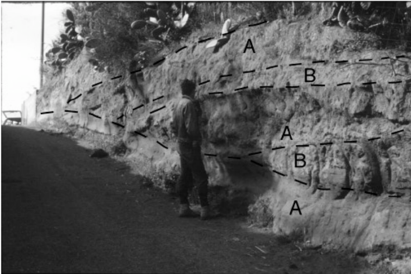
Fig. 3 TGR inf. sequence in the Piano area. A lithofacies-A layers with concavo-convex bedding planes; B lithofacies-B layers. The dashed lines mark the contact between different lithofacies
