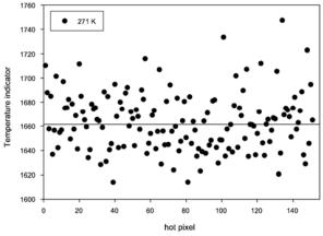
Fig. 2. Temperature indicators for a dark frame taken at 271 K.
