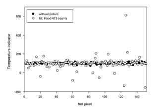
Fig. 5. Temperature indicators for the image of Mt. Hood normalized to 413 counts plus a dark frame taken at  $242~\mathrm{K}$ .
