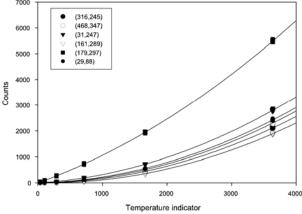
Fig. 1. Counts versus temperature indicator for 6 different pixels.
